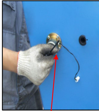
Electromagnet on the outer surface of the column
