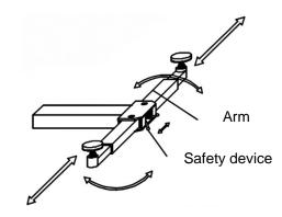
You can adjust the support arms as follows: Pull the safety bolts, you can now adjust the support arms, Release the safety latches to lock the support arm.
