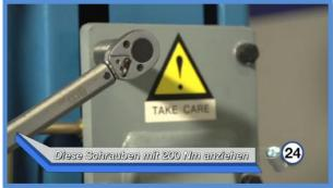
These screws must be tightened with a torque of also 200 Newton meters crosswise. Thus, the assembly is almost complete.
