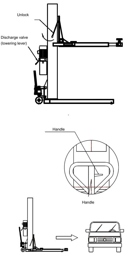
Put the mobile 1 Colum lift under the vehicle
