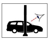
After a short lifting, check the vehicle for a secure fit!
