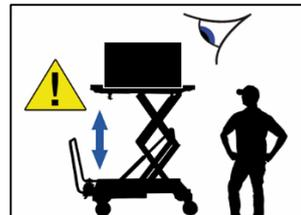
Always monitor the scissor lift table (when lifting or lowering)!
